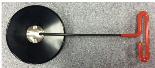
\frac{1}{8} " T-wrench inserted into the adjustable screw
