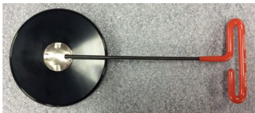
\frac{1}{8} " T-wrench inserted into the adjustable screw
