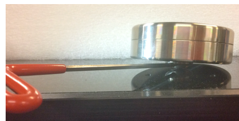
Adjusting the V-150A model using a 1/8" T-wrench
