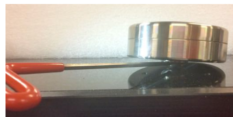
Adjusting the V-150R model using a 1/8" T-wrench
